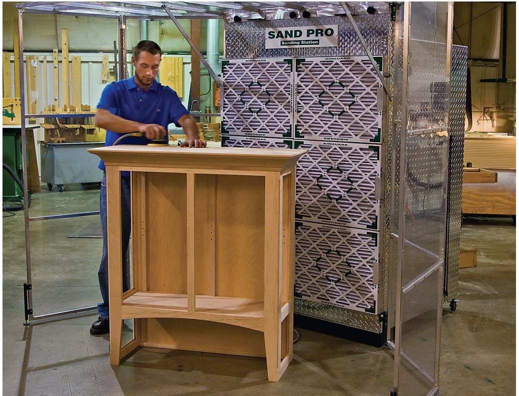
The Sand Pro sanding booth, model SB108, features hinged vinyl sides and top panels to construct the best perimeter for your workpiece, up to 9' wide.
